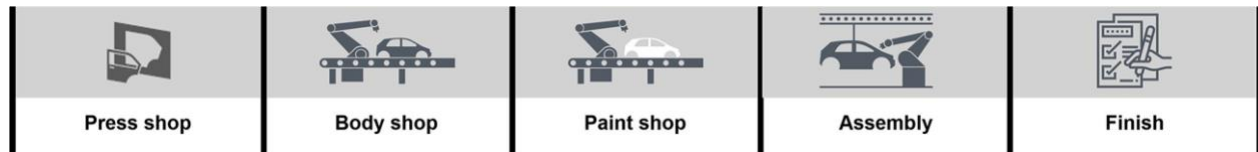
Figure 3: Vehicle manufacturing process (Demlehner et al., 2021: 3)
